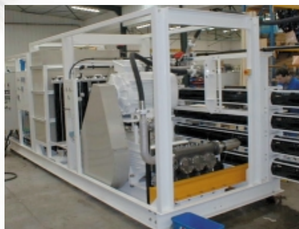
150 Frame Salt Water Reverse Osmosis Systems
