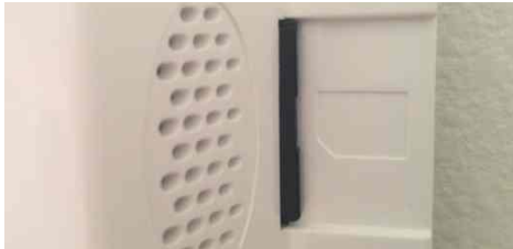
Card will slide all the way in. To remove, push gently and card will spring out.
