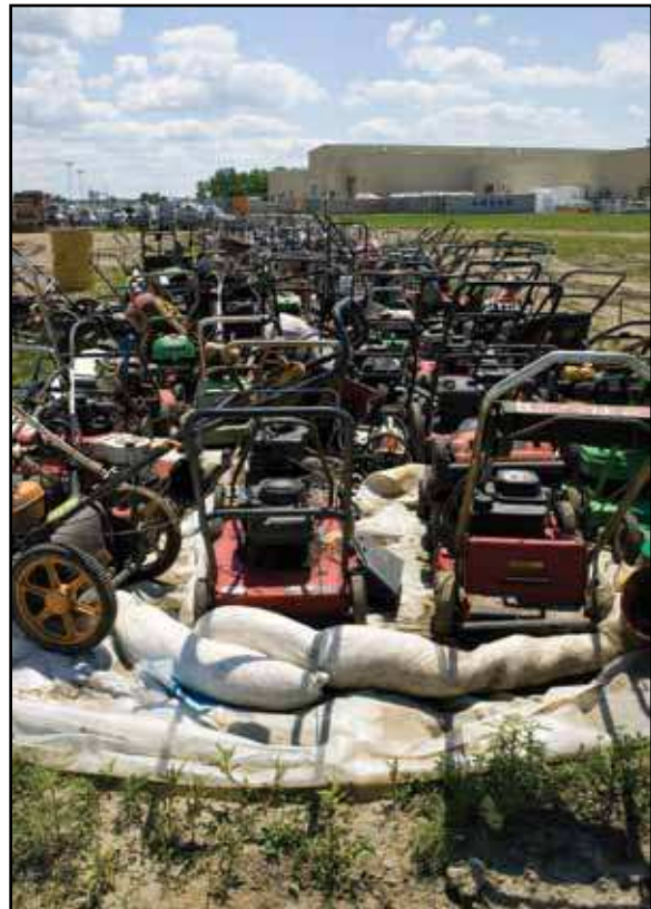
Figure 3: Segregation of hazardous debris
