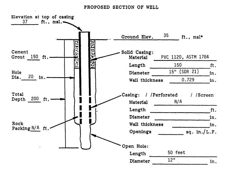
\*Approximate elevation at time of filing application. Final elevation (msl) by a surveyor licensed by the State must be submitted at start of construction.
