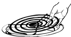
Lift the surface unit about 1 inch above the drip pan and pull it out.
