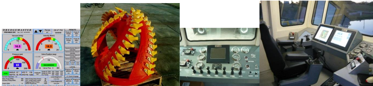
Dredge Panel-GPS Business end of dredge Dredge Controls Dredge Control Cab
