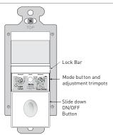
To access mode button and adjustment trimpots, gently pull the Lock Bar away from the switch face and slide the ON/OFF button
