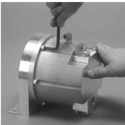
Step 6. Figure 6 Using a 6mm (1/4") hex head wrench, remove the liquid chamber bolts that connect the chamber cover to the liquid chamber.
