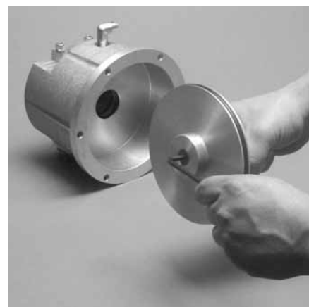
Step 10. Figure 10 Using a 5mm (3/16") hex head wrench, remove the liquid piston from the power piston by turning the power piston screw counter-clockwise.
