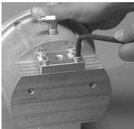
Step 15. Figure 15 To inspect or replace the discharge manifold O-ring, valve seat O-ring, valve seat, valve ball and ball cage, first remove the combo manifold plate located at the top of the liquid chamber. To inspect or replace the inlet manifold O-ring, valve seat O-ring, valve seat, valve ball and ball cage, repeat process.
