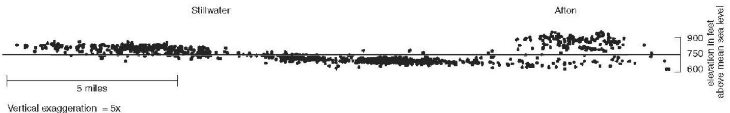
Figure 2. North to south cross section showing Jordan Sandstone top elevations from the County Well Index water well database in the Stillwater/Afton area. Elevation change for the top of the Jordan Sandstone is over 300 feet. The large spread of top elevation around the Afton area reflects projection of data that include wells on both upthrown and downthrown sides of faults.
