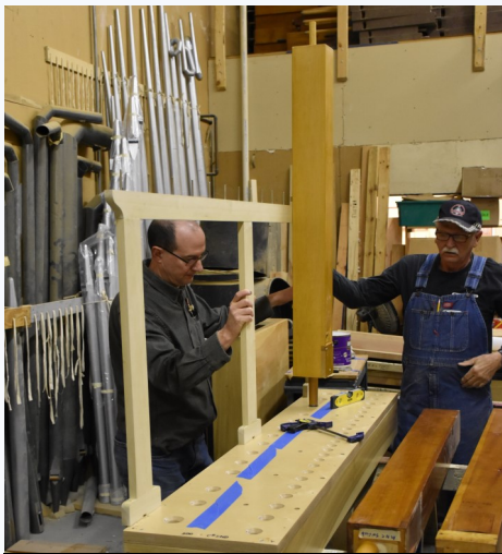
Two of Dan Garland's shop workers insert a wooden pipe into a pipe rack that is part of MPC's organ
