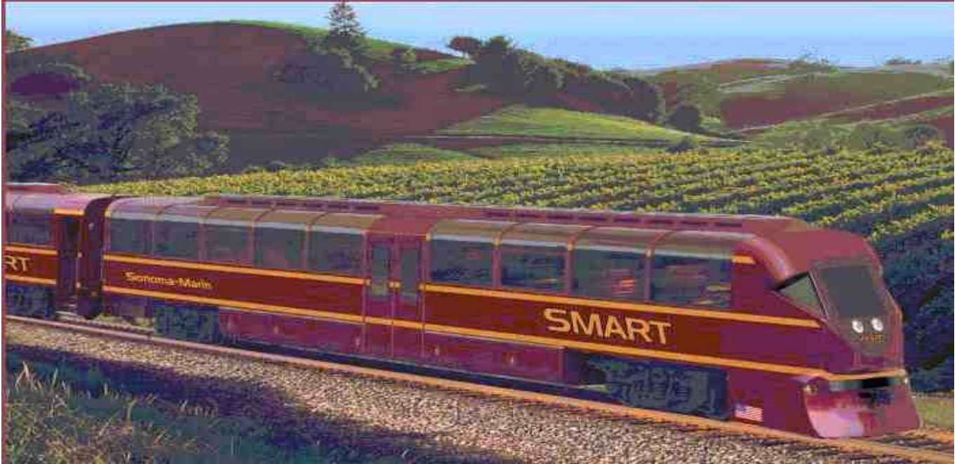
Proposed Diesel Multiple Unit to be used in 3 car trains. Vehicle can be run on bio-diesel.
