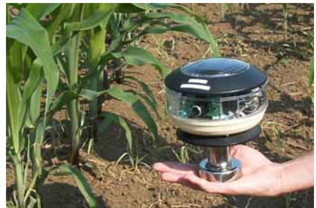
Fig.1. Field Server as a Web-based sensor node.
