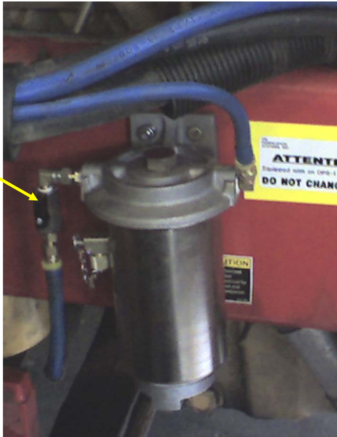
Figure 8 – Location of Shut-off Valve on the Filter
