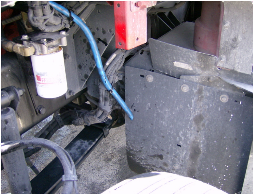
Figure 7 – Venting Hose Termination
