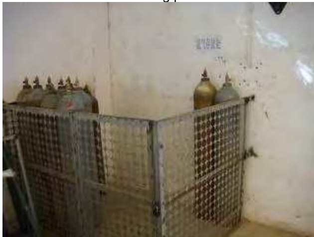
Hazard storage inside workshop(with cage and secondary container)
