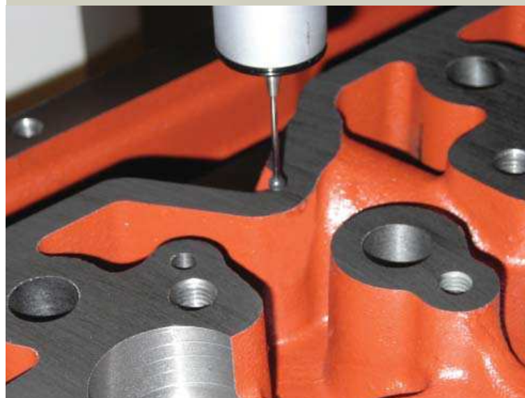
Cummins runs many touch sensor inspection tasks, including the scanning of surface valve cover sealing.
