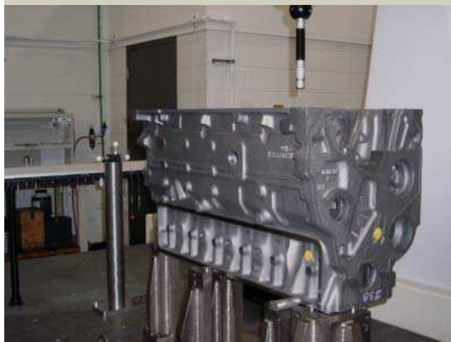
RMEP's non-stop metrology operations dedicate 4 Metris CMMs to cylinder block scanning.
