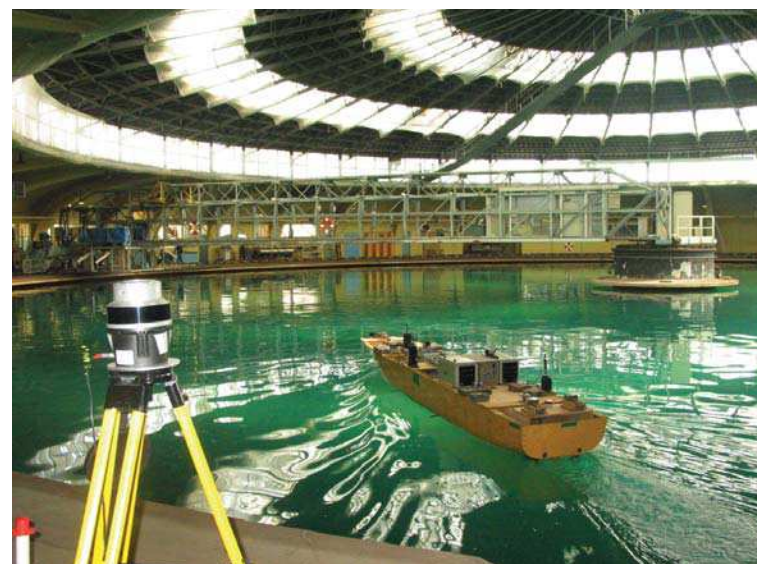
The transmitters around the gyration tank activate a metrology-enabled area that spans the entire tank.
