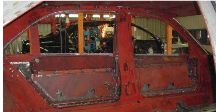
Reverse engineered steel armoring parts make up a bullet-tight cage around the interior of a vehicle body.
