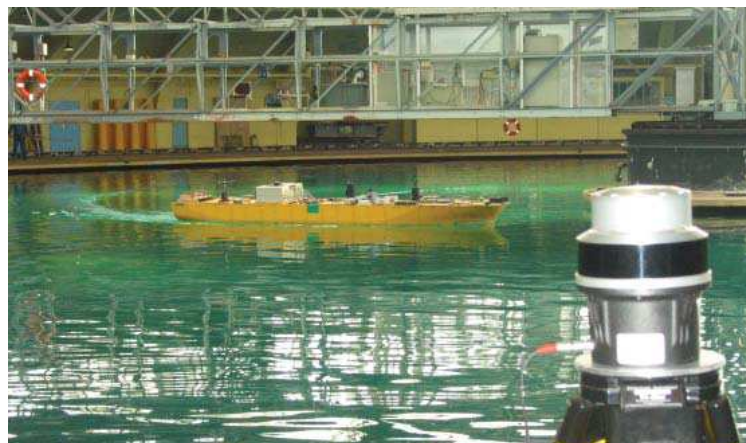
Metris iGPS accurately measures the boat trajectory by dynamically and concurrently acquiring sensor data.
