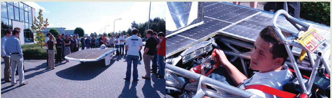
This one-seater only weighs 175 kg and features dynamic wind resistance that is roughly six times better than premium serial-produced sports cars.
