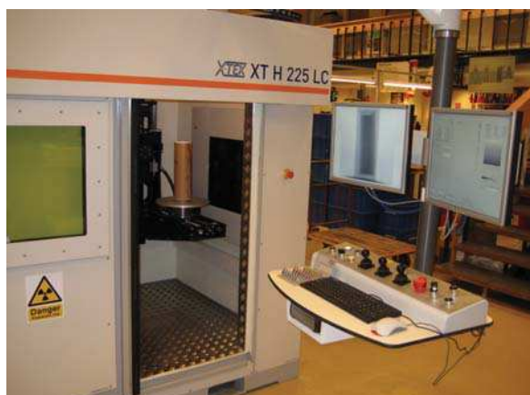
A smaller sample installed for inspection
