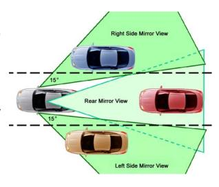
overlap between the inside and side-view mirrors and **allows the driver to monitor the adjacent lane**. Traditional settings overlap with the rearview mirror view and should only be used if the view of the highway from the inside rear-view mirror is blocked.
