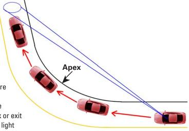
The vehicle's speed and load, and the sharpness and bank of the curve effect vehicle control. Traction loss when entering a curve is often caused by excessive speed, braking, or steering. Front tire traction loss is referred to as "under-steer," and is more likely to occur in front-wheel drive vehicles. "Over-steer" is when there is traction loss by the rear tires and occurs more often in vehicles with rear-wheel drive.
