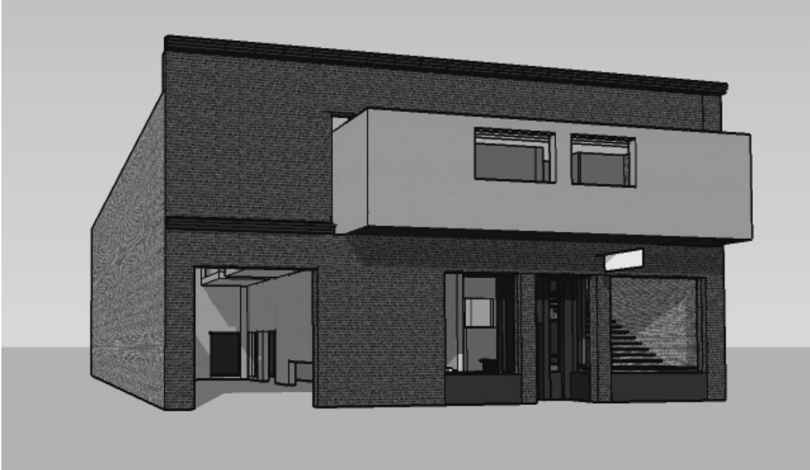
Figure 12: Massing Model using SketchUp. Notice that each hotel room protrudes through the structural wall, looking down upon the courtyard or sidewalk.
