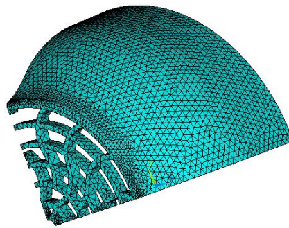
Figure 12. Fan cover finite element model.
