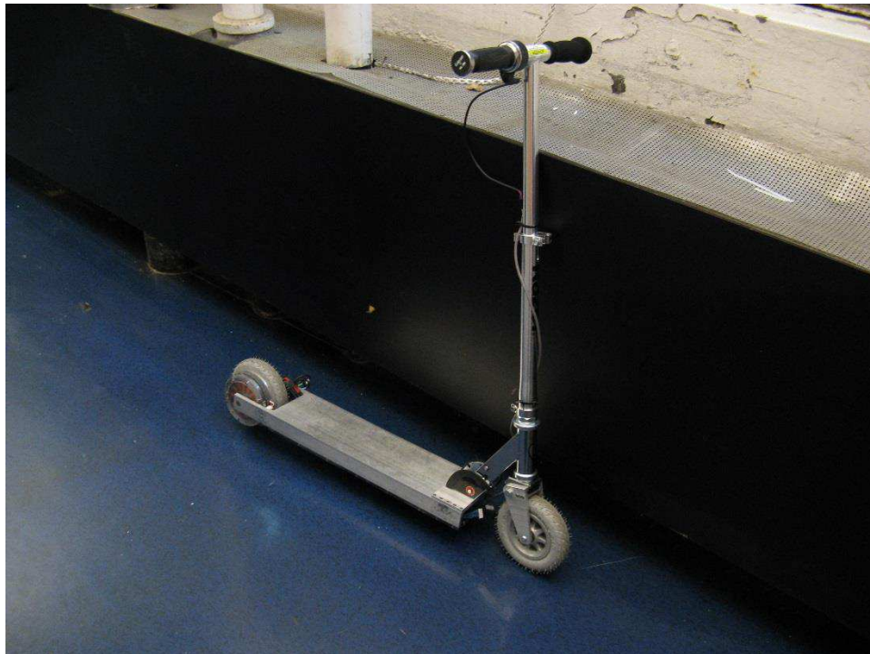
Figure 37: Pneu Scooter, a lightweight electric kick-scooter with a custom in-wheel motor.
