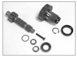
Complete SportGear kit, above, features a lengthened output shaft (main gear) with an integral retainer ring to keep the oil seal from falling out of the bore – a common problem with OEM and other aftermarket parts.
