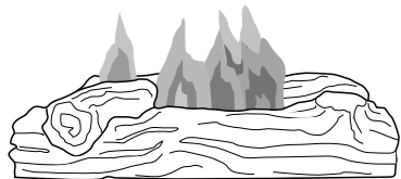
Figure 32 - Incorrect Burner Flame Pattern
