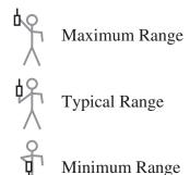
If your finger touches the antenna near the dial on the top of the transmitter, the actual range may be reduced. Additional environmental factors may also affect the range of your unit.
