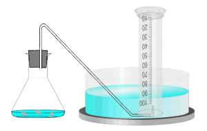
The easiest and most common method is to collect the *gas* in an upturned *measuring cylinder* filled with *water*.
