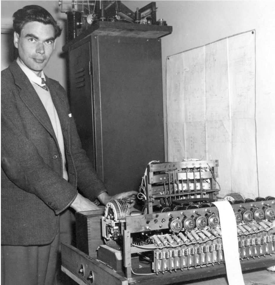
Figure 3: 'The recording device shown in the photograph, which I called Thoth, after the Egyptian god of writing and wisdom, was built to record the results (which were signalled with electrical contacts on the escape controls) of the simulation of a disabled submarine. It was based on a pallenotype machine, with a keyboard and the letters of the alphabet – used for shorthand. In front of the curved strips (below the vertical push rods) was the keyboard working the pallenotype. Unlike a typewriter any number of keys could be pressed at once. To the left is a clock, in the box, which was used by RAF fighter command for allocating 15-second periods for transmission and reception with four different “coloured” squadrons sending pulses to the uni-selector – which is the curved object in front of the box. This part was from telephone exchanges - we used whatever we could get hold of – and was wired up to code letter keys to indicate time, I think to the nearest second. The experiment lasted ten hours. Later I redesigned the time system using a mechanical counter like the mileometer on a car, with the typeface on the wheels, which printed time in numbers. This was quicker to read. The device was then made a lot smaller and neater, later manufactured by the Cambridge Instrument Company. It was not a total success as it was not entirely reliable, but it was a start towards automatic recording.' Professor Richard Gregory, 3 and 5 December 2002.
