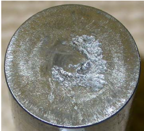
Figure 5. Spalling on Lifter Face, Abnormal Condition
