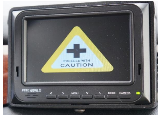
Figure 33. Close up of Proceed with Caution on in-vehicle display
