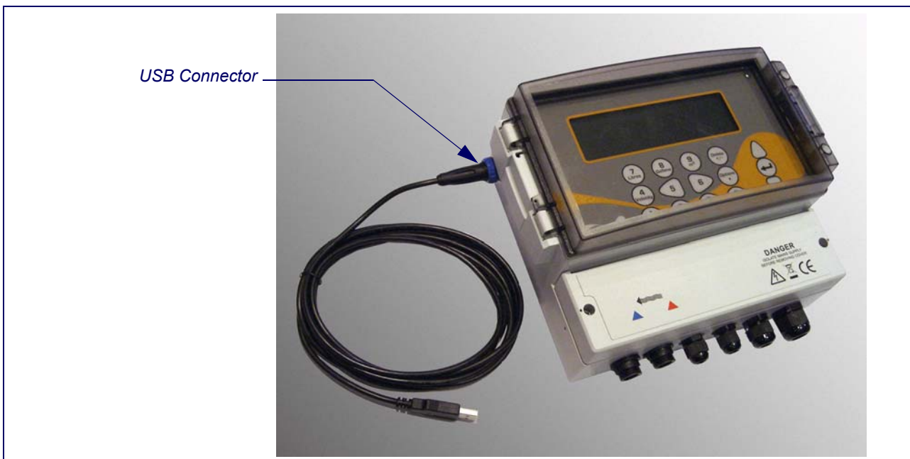
Figure 2.2 U4000 USB Connection
