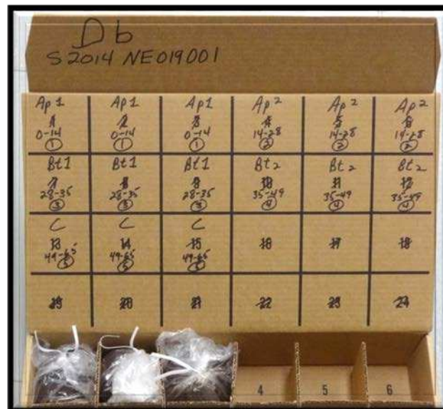
Figure 9.—The inside of a correctly labeled clod box. Each cell is labeled. (Step 20)
