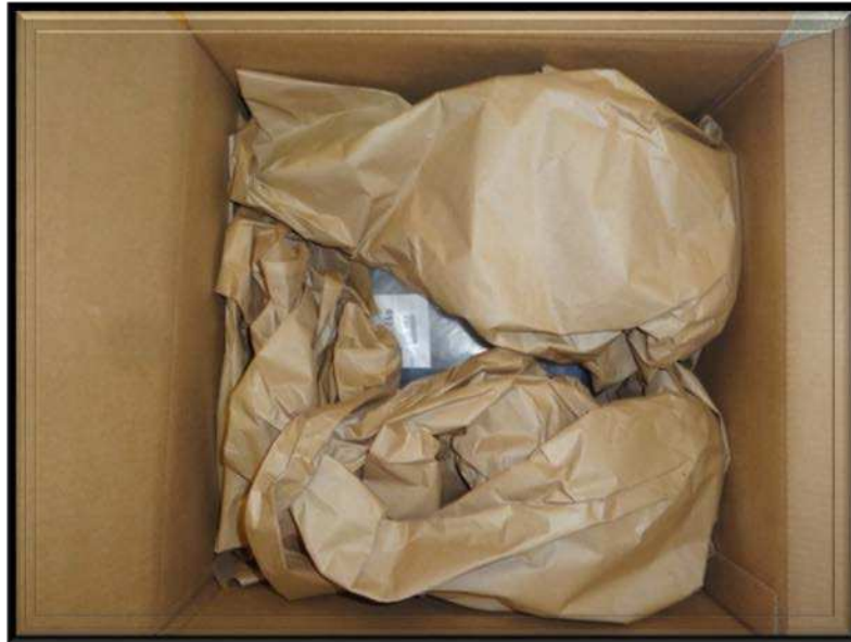
Figure 6.—Packing material used to stabilize the bulk sample in the cardboard box. (Step 13)
