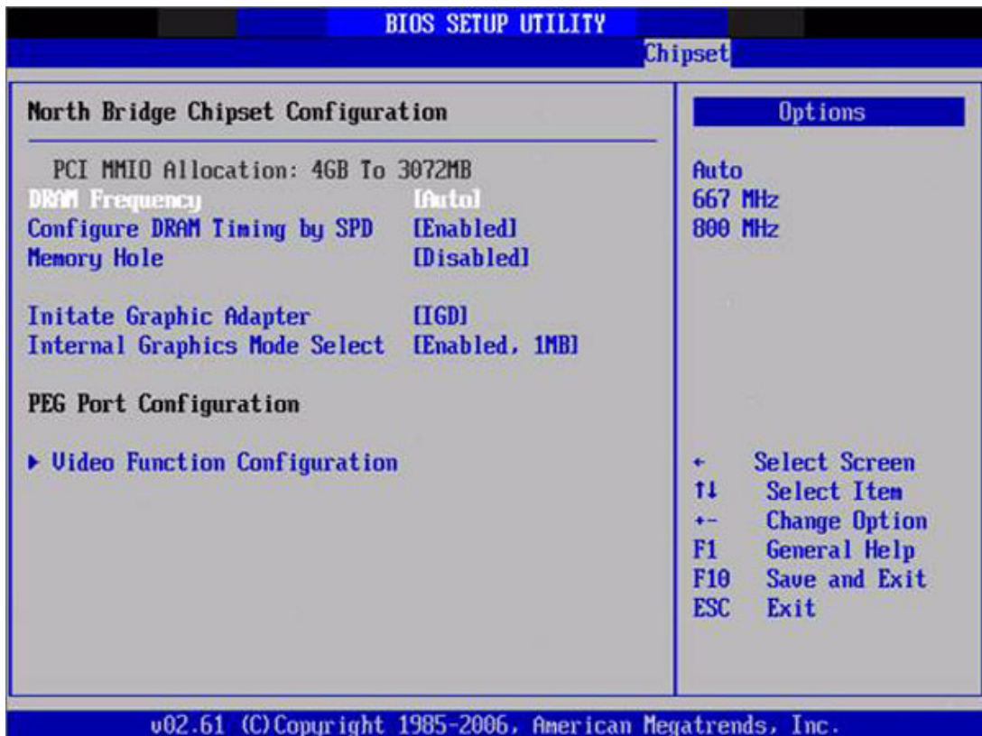
Figure 3.24 North Bridge Configuration
