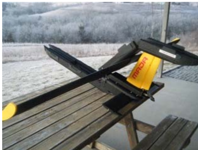
Note that the fuselage can be opened for convenient work on electrical components, and installation of cameras and video recorders.
