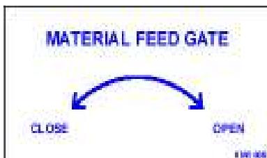
Opens and closes the material feed gate which in turn controls the production.
