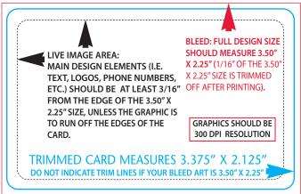
LIVE: 3.125" x 1.875" major design elements should be placed within the "Live" image area. BLEED: 3.50" x 2.25" all items that run off the card must reach the "Bleed: size/edges. Do not cut off corners of art.
