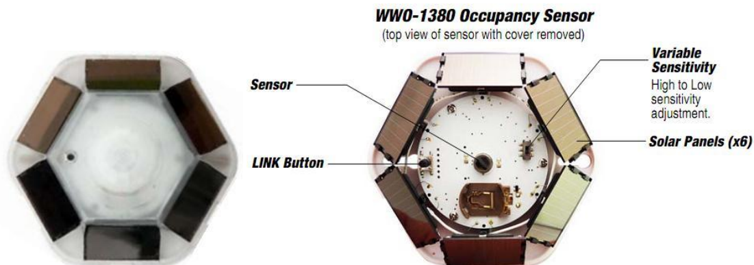
Figure 5.5 – Wireless, solar-powered occupancy sensor (Douglas Lighting Controls, 2011)
