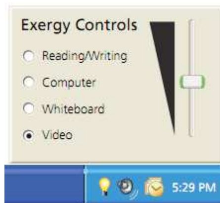
Figure 5.11 – Example of personal computer lighting control software (Exergy Controls, 2009)
