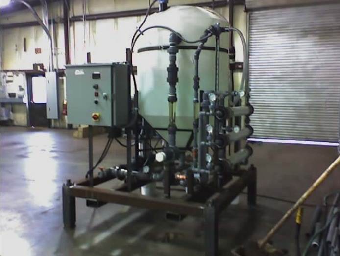
Figure 4. Steward Environmental Solutions 10 gpm continuous flow SAMMS® filtration system.
