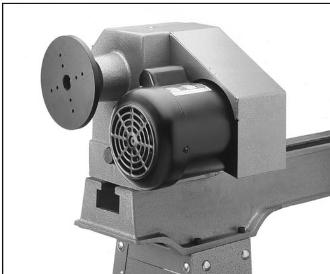
Figure 25. Headstock set at 180°.
