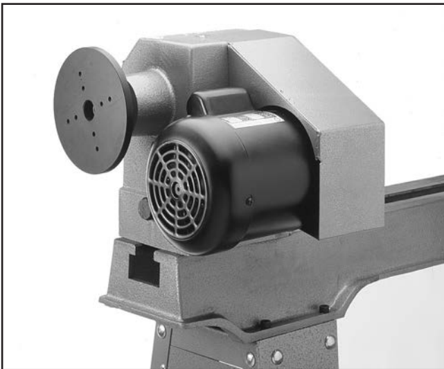
Figure 17. Headstock set at 180°.
