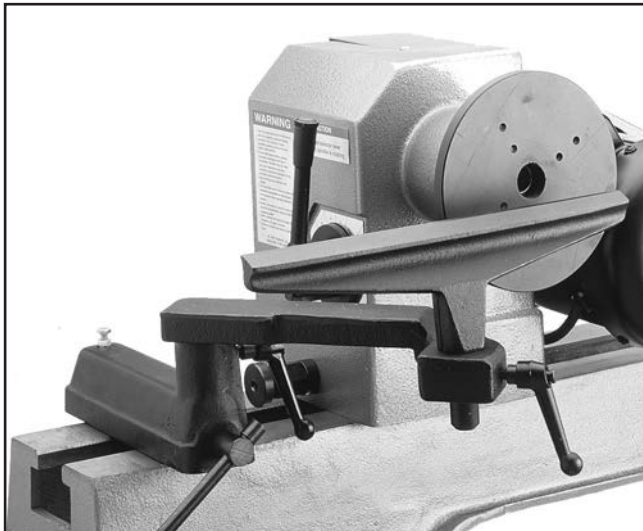
Figure 24. Headstock set at 90°.
