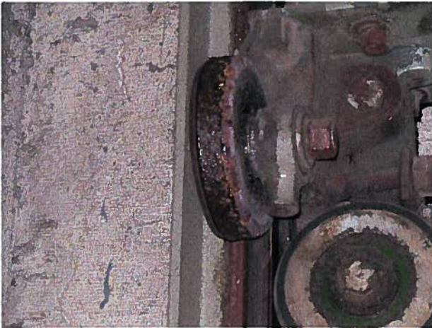
WORN COUNTERWEIGHT ROLLER
