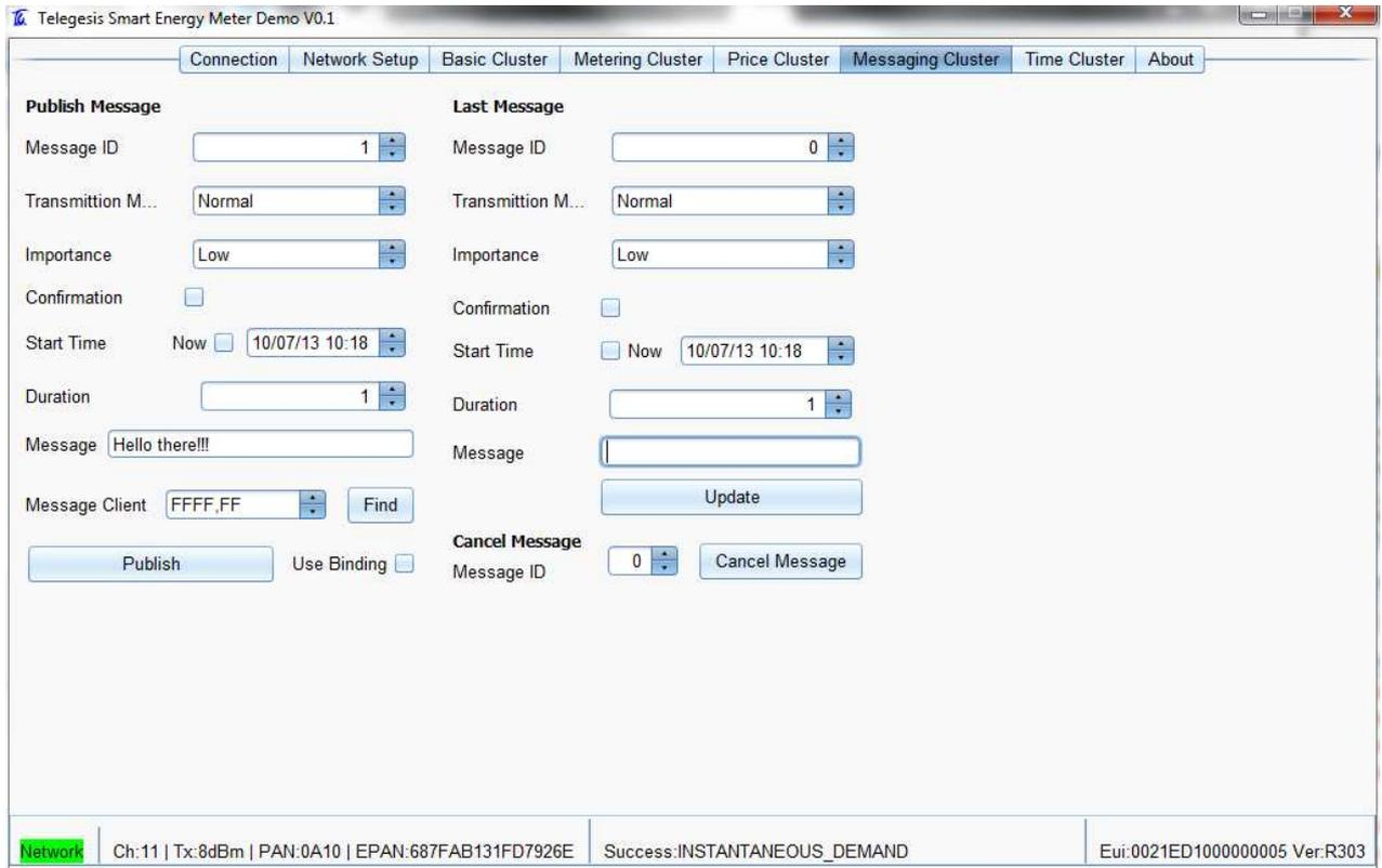
Fill in the required fields appropriately in compliance with the ZSE1.1 specification and publish the message using either “Use Binding” to send to all Messaging Clients listed in the binding table or to an individual Message Client by either discovering it using “Find” or by supplying its node ID and endpoint and then clicking the “Publish” button.
