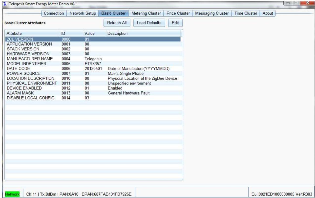
The screenshot shows the 'Basic Cluster Attributes' window in the Telegesis Smart Energy Meter Demo V0.1 application. The window has tabs for Connection, Network Setup, Basic Cluster (selected), Metering Cluster, Price Cluster, Messaging Cluster, Time Cluster, and About. Below the tabs are buttons for Refresh All, Load Defaults, and Edit. The main area contains a table with the following data:
