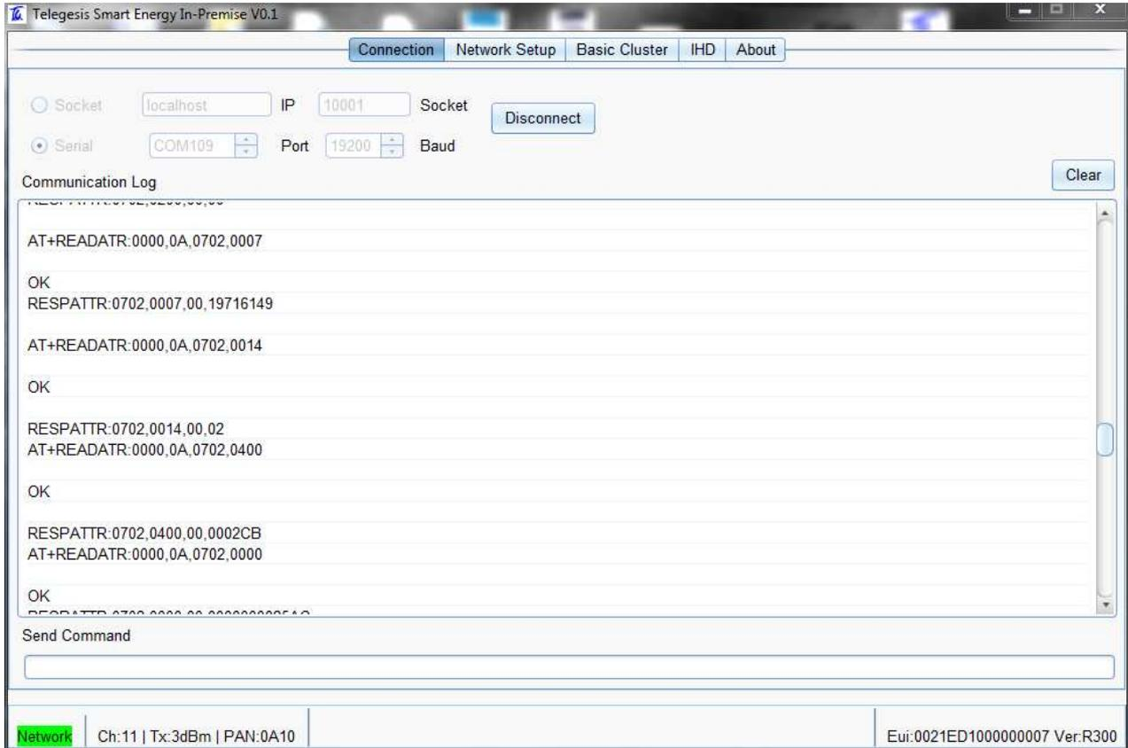
If the selected Serial Port does not connect to a IPD ETRX3USB then an error is shown in the status bar.
