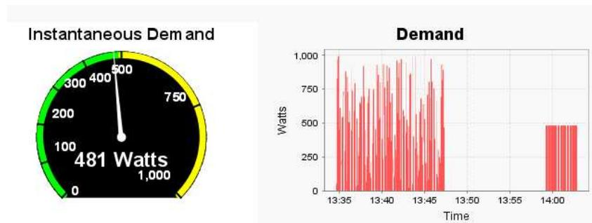
This part shows the Instantaneous Demand attribute as received from Mock Meter ETRX3USB as a meter dial as well as plotted in a chart against time. This visualization is updated periodically at an interval of 5 seconds.
