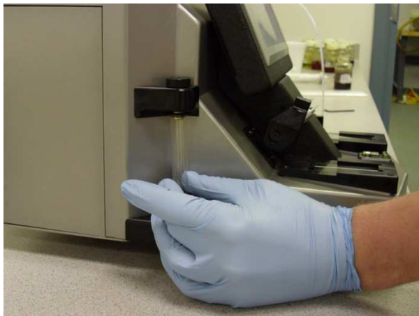
Figure 8.1 – Installing Sample Vial
