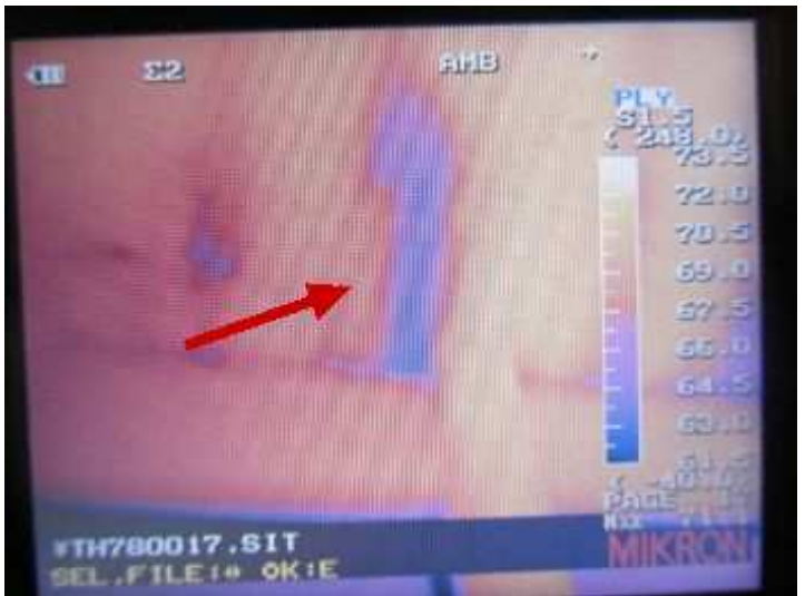
There are two areas on the ceiling where cold spots where detected with the thermal infrared camera, check with moisture meter reading were 5% moisture no moisture present in the cold spots on the ceiling.
