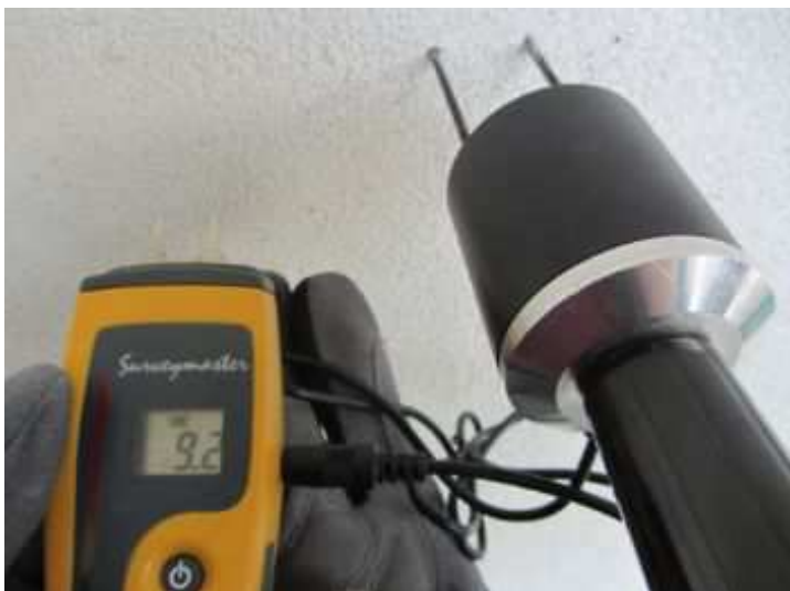
Baseline moisture level from the moisture probe test in dry area was between 7.5% to 9.2% moisture.
