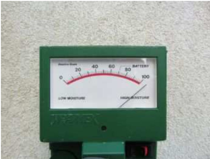
Tramex wet wall detector reading 100%
