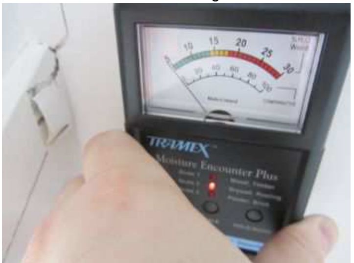
There are two areas on the ceiling where cold spots where detected with the thermal infrared camera, check with moisture meter reading were 5% moisture no moisture present in the cold spots on the ceiling.
