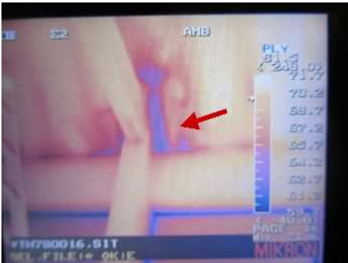
There are two areas on the ceiling where cold spots where detected with the thermal infrared camera, check with moisture meter reading were 5% moisture no moisture present in the cold spots on the ceiling.
