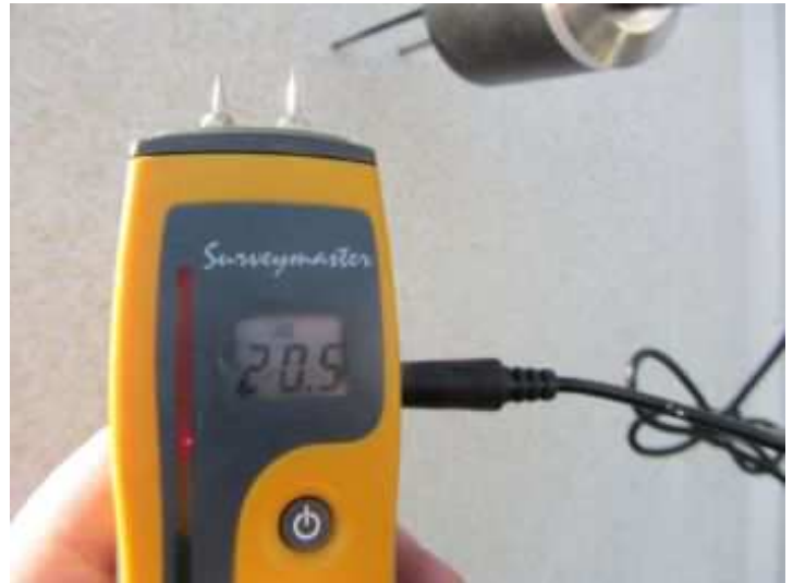
GE Surveymaster moisture meter probe reading between 20.5% moisture.
