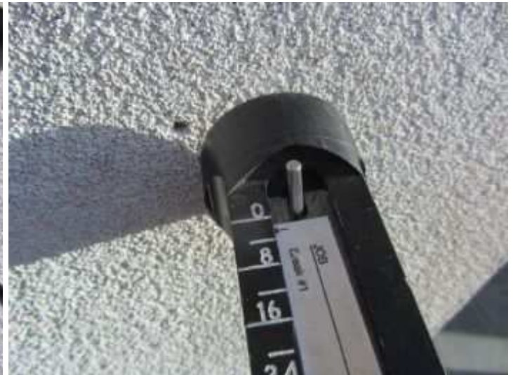
The substrate resistance tester(SRT) measure less then 5 pounds of resistance when popping through the wood substrate on a small area in the front elevation.
