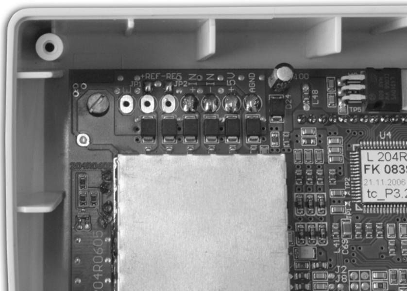
The contact tabs for the weighing cell are positioned on the top left-hand corner of the board.
