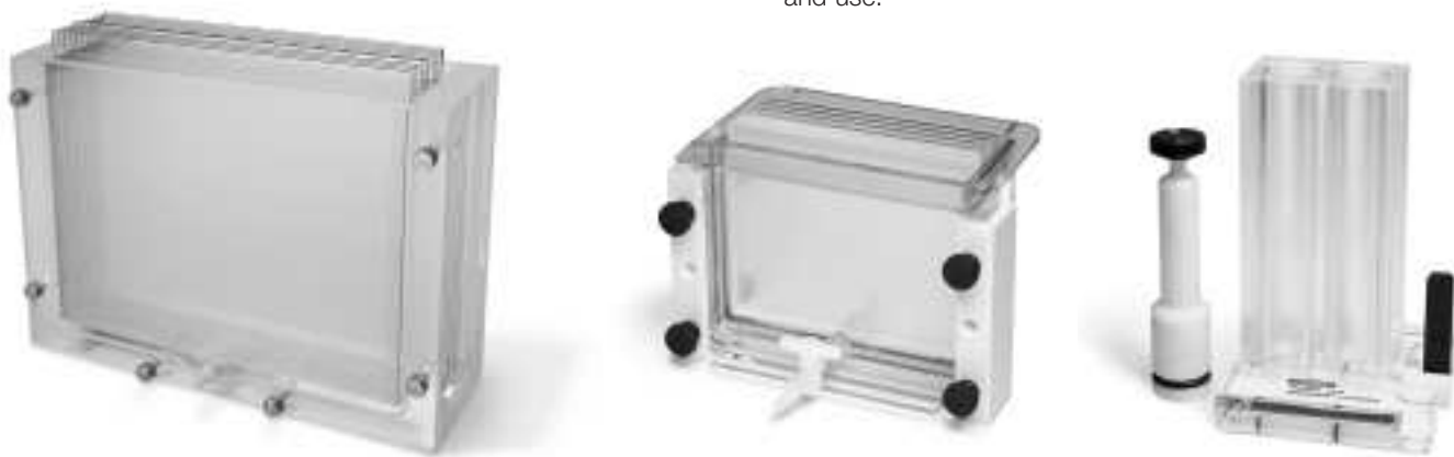
Fig. 11.1. Apparatus for casting multiple gels. Multi-casting chambers for 12 PROTEAN Plus™ 3 gels or for 12 Mini-PROTEAN® gels allow uniform casting of gradient gels. Gradient makers are available for both size formats.
