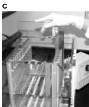
Fig. 11.3 C. A gel is being inserted into the PROTEAN Plus Dodeca cell. The top of the gel is aligned with the agarose-embedded IPG strip at the cathode (negative electrode) side of the tank. This cell accommodates PROTEAN XL Ready Gel precast gels (shown), or PROTEAN Plus handcast gels up to 25 cm wide. A uniform electrical field is applied via metal plates. The pump visible behind the tank circulates the buffer to maintain a uniform temperature during the run.
