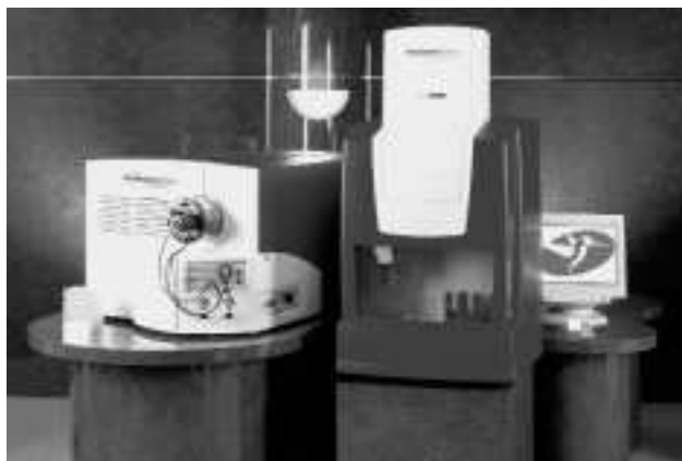
Fig. 8.4. M@LDI HT, the "2-D gel-MS" analyzer of the ProteomeWorks System. Q-ToF micro with capillary HPLC optimized for high-sensitivity LC-MS-MS in post-genomic studies.
