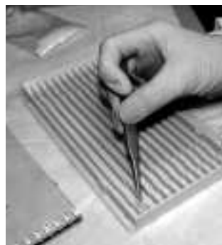
Fig. 10.2. Placement of wicks on the electrodes in each channel that will be used. IPG strips will be placed on top of the wicks.
