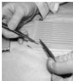
Fig. 10.3. Insertion of wicks under both ends of an IPG strip that has been rehydrated in a focusing tray.
