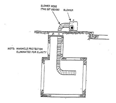
DURING VENTILATION ONLY TWO 90° BENDS ARE PERMITTED IN THE BLOWER HOSE AND THE END MUST BE SECURED IN A HORIZONTAL POSITION DIRECTED TOWARD AN END WALL OF THE SPACE.
