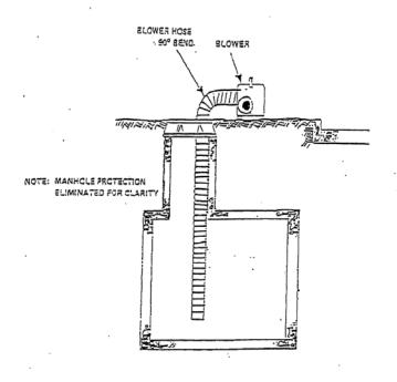
DURING PURGING ONLY ONE 90° BEND IS PERMITTED IN THE BLOWER HOSE AND THE END MUST POINT DOWN AND REACH NEAR THE BOTTOM OF THE SPACE.
