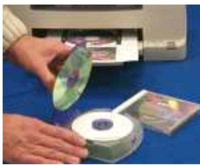
5) Remove CD label from the form. Use a standard CD label applicator to properly adhere label to CD.
