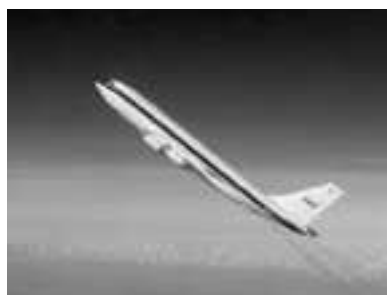
The Vomit Comet is a modified KC-135 tanker. It flies a parabolic flight path, giving 25 seconds of weightlessness. Pictures courtesy John Hopkins University and Asher Langton - University of Wisconsin Madison.
