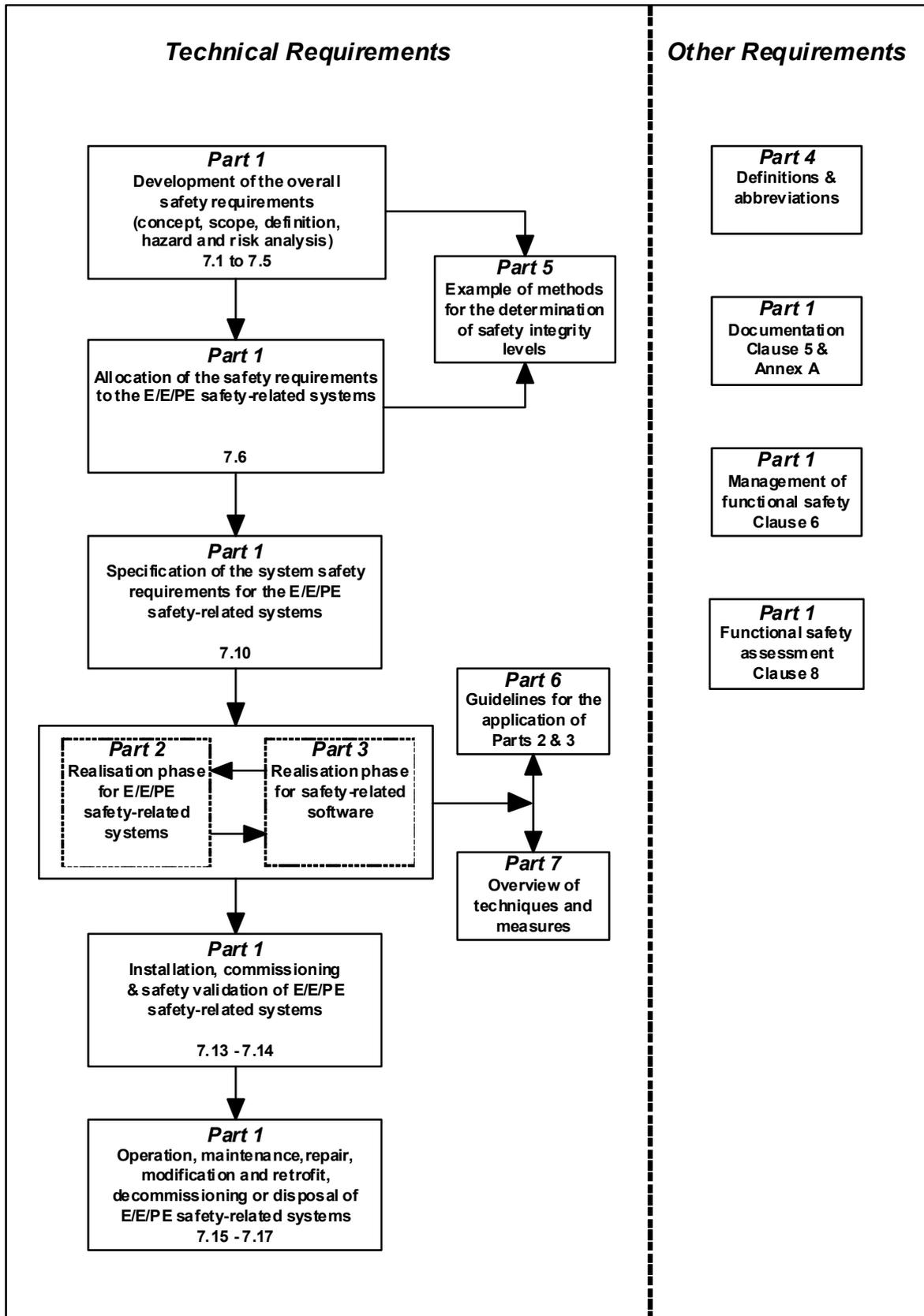
Figure 1 – Overall framework of the IEC 61508 series
