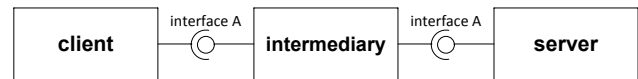
Figure 4: An instrumented connector has an intermediary component in the connection between client and server.
