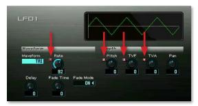
In this patch editing example, we're editing an LFO, where the Rate, Pitch, TVF, and TVA parameters can be set using Knobs 1-4, respectively.
