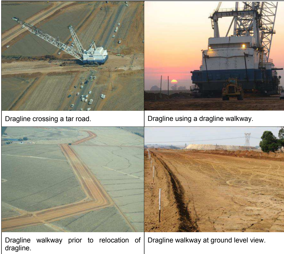
Image 1-2: Photographs depicting typical dragline relocations.
