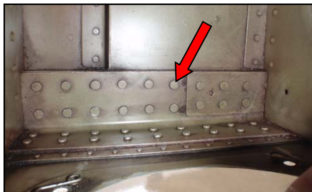
FIG. 7. PRE-MODIFICATION H.289 RIVETED ATTACHMENT OF ALUMINIUM ALLOY INSERTS
