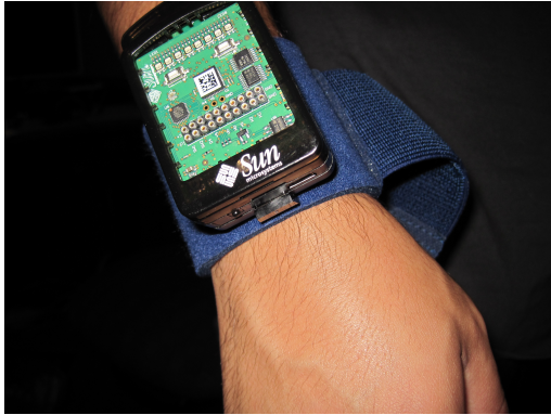
Figure 4: SunSPOTs are worn on the wrist and the thigh. Each node samples the corresponding accelerometer values.
