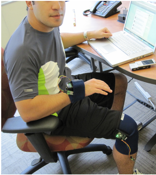
Figure 1: TwitterJacket takes advantage of accelerometers on the thigh and the wrist as well as an ECG monitoring t-shirt to observe user activity and health and report the results on Twitter.
